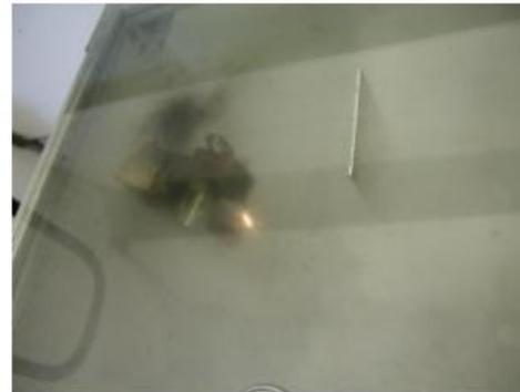
Controlled Class A flame in space shuttle mid-deck locker (Abbud-Madrid et al. Colorado School of Mines, CSM)
