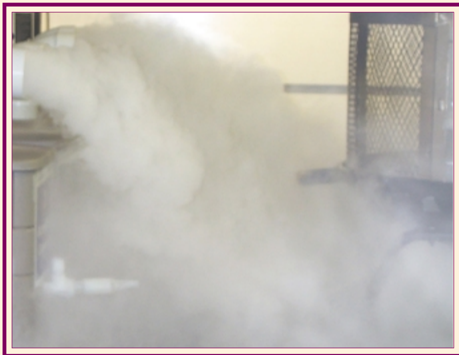
Figure 1. A dense gas-like ultra fine water fog (NanoMist) dispersion in a room
