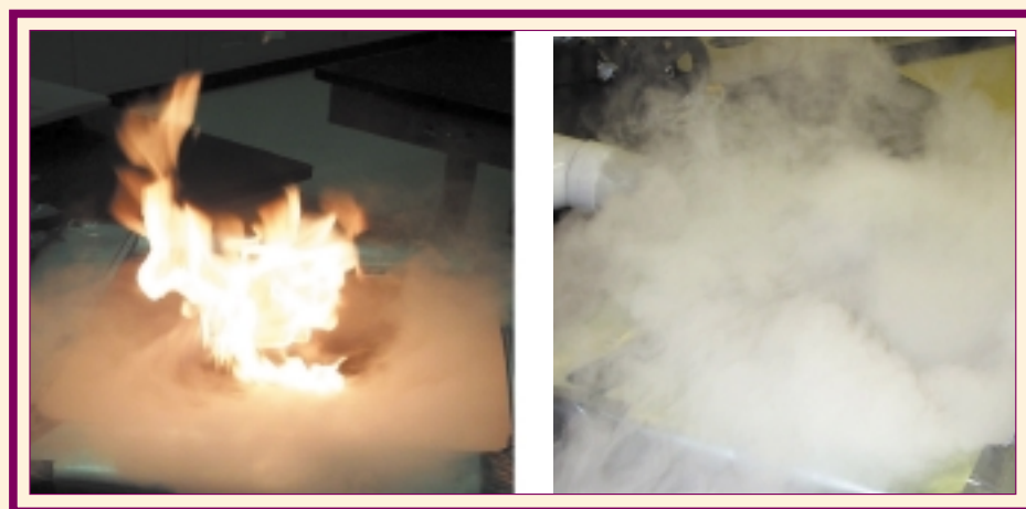
Figure 8. A special configuration of heptane liquid pool fire suppression where NanoMist surrounds the firebase
